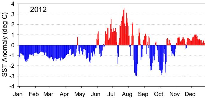
**Figure 5.** Daily SST anomalies at NOAA Buoy 46050, off Newport, Oregon showing the extended period of warm water observed during the summer of 2012. Both June and July were considerable warmer than normal.
