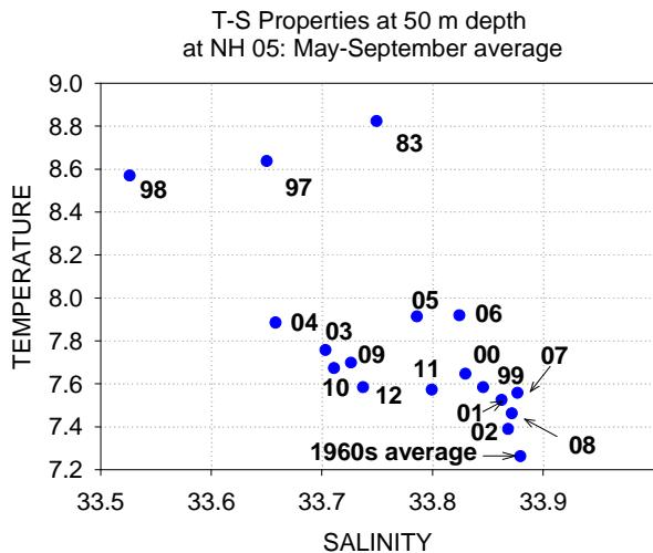
**Figure 9.** Temperature and salinity values measured at a depth of 50 m at station NH05, off Newport, OR over May-September. These values can be viewed as a measure of upwelling strength – e.g., cold and salty values indicate strong upwelling. The summer of 2012 was relatively cool compared to other years (averaged 7.58°C) but considerably fresher (33.738).
