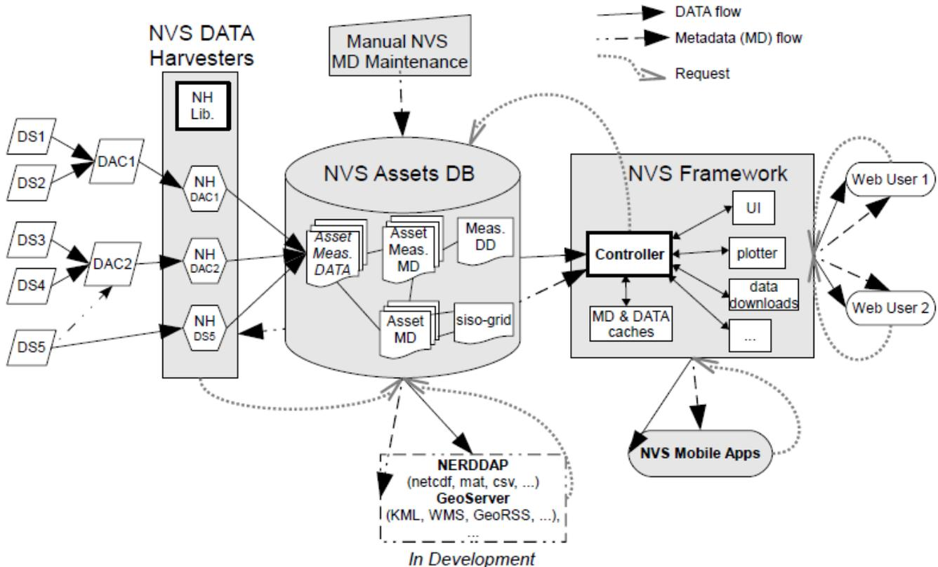
**Fig. 1.** NVS Information System Schematics. Shaded blocks represent broad NVS components. The dashed DS5-DAC2 arrow represents an alternate access point for DS5 assets. Acronyms and abbreviations used: DAC (Data Assembly Center), DD (Data Dictionary), DS (Data Source), Lib. (Library), MD (Metadata), Meas. (Measurements), NH (NVS Harvester), UI (User Interface).
