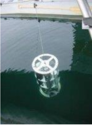
CTD being lowered through trap door of float plane into the water
