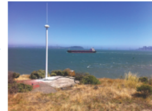
Figure 1. IOOS operates the nation's only network of land-based high-frequency radars (pictured above) that provide continuous, real-time mapping of the speed and direction of surface currents in coastal waters.
