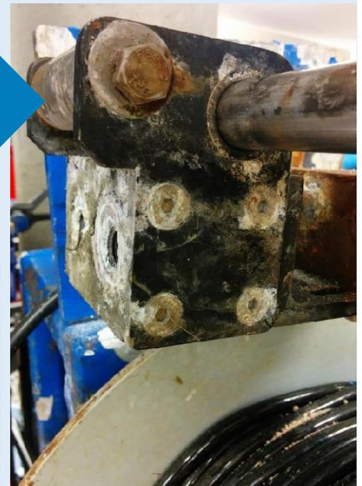
Vital buoy winch parts wear out from being in a seawater environment 24 x 7 x 365
