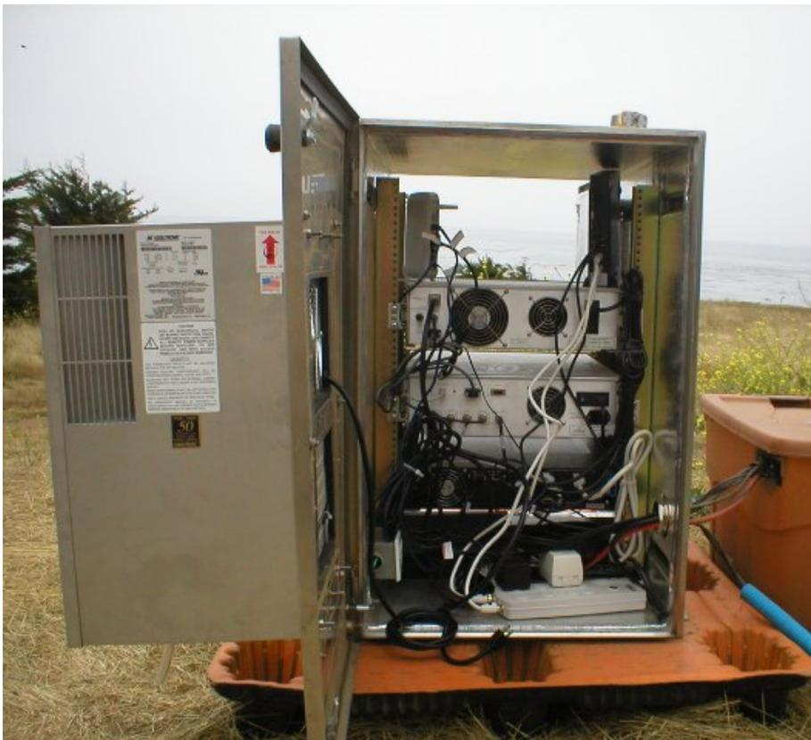
Figure 2. View of outdoor electronics enclosure with both doors open. Air conditioner is attached and all HFR electronics are mounted within the enclosure.
