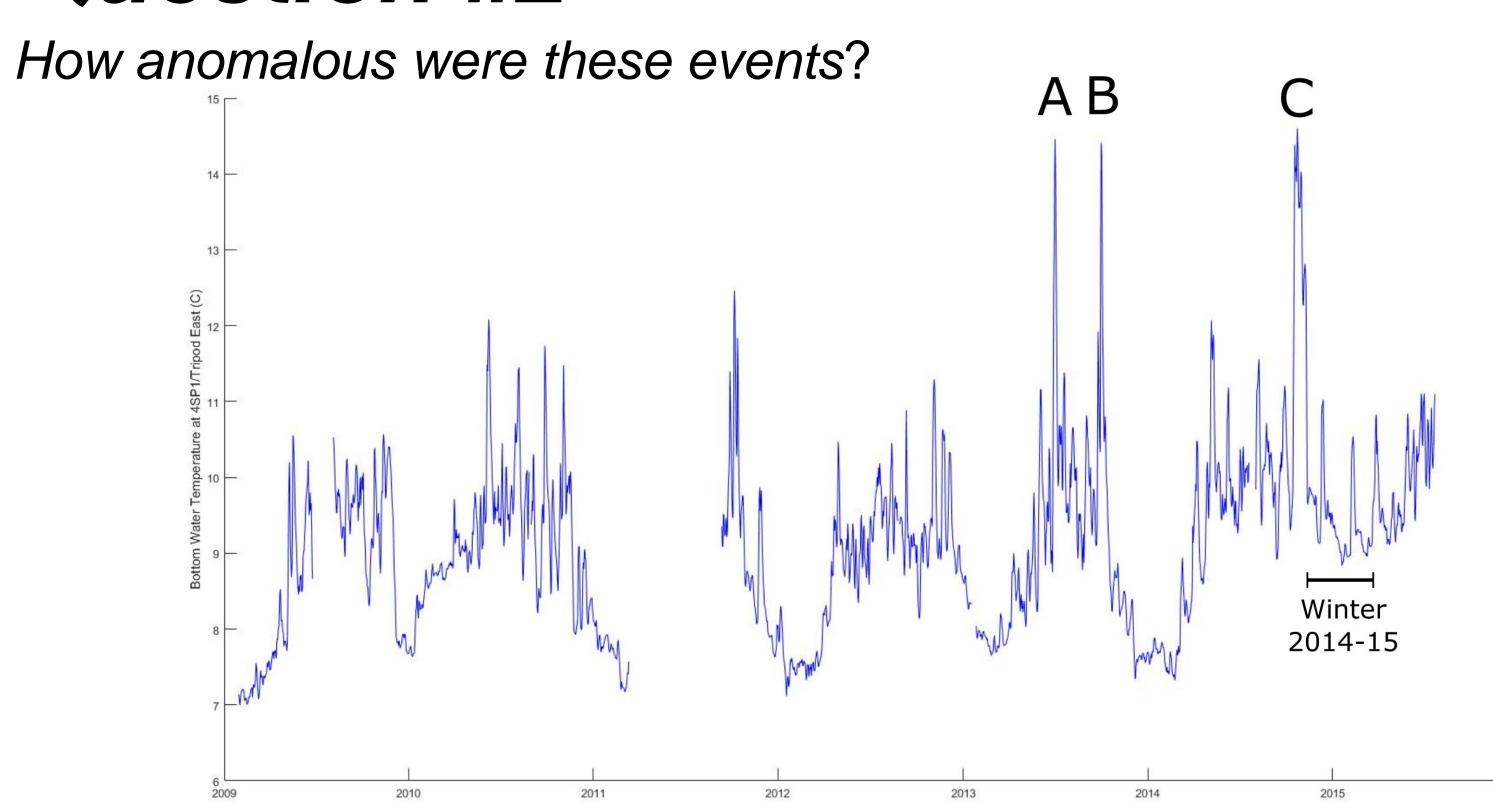
Coupling HOBO data collected between 2011-2015 from a site at Elwha at ~6m depth with temperature data collected using a Seabird SB26+ pressure sensor deployed at the same location from early 2009-2011, a longer time-series is developed (above). These three events were associated with temperatures ~2C higher than anything in the record
