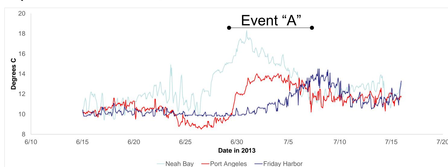
The timing of elevated surface water temperature at two NOAA tide stations (Neah Bay and Friday Harbor; see map at upper left) relative to event "A" suggests that the warm water propagated into the Strait from offshore.
