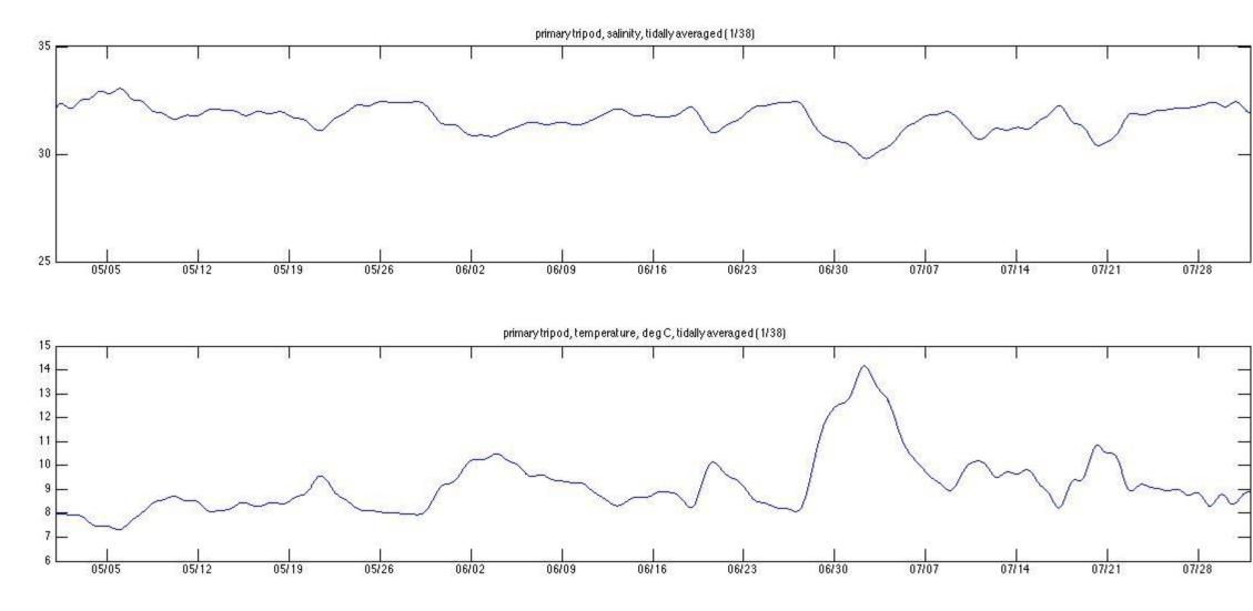
Tidally-averaged temperature and salinity from a CTD at 15m depth and ~1000 m north of the Elwha River mouth suggest that event "A" was associated with lower salinity (see above), but all three events were recorded by a HOBO near Green Point (see below) at ~18m depth and distant from a freshwater source.
